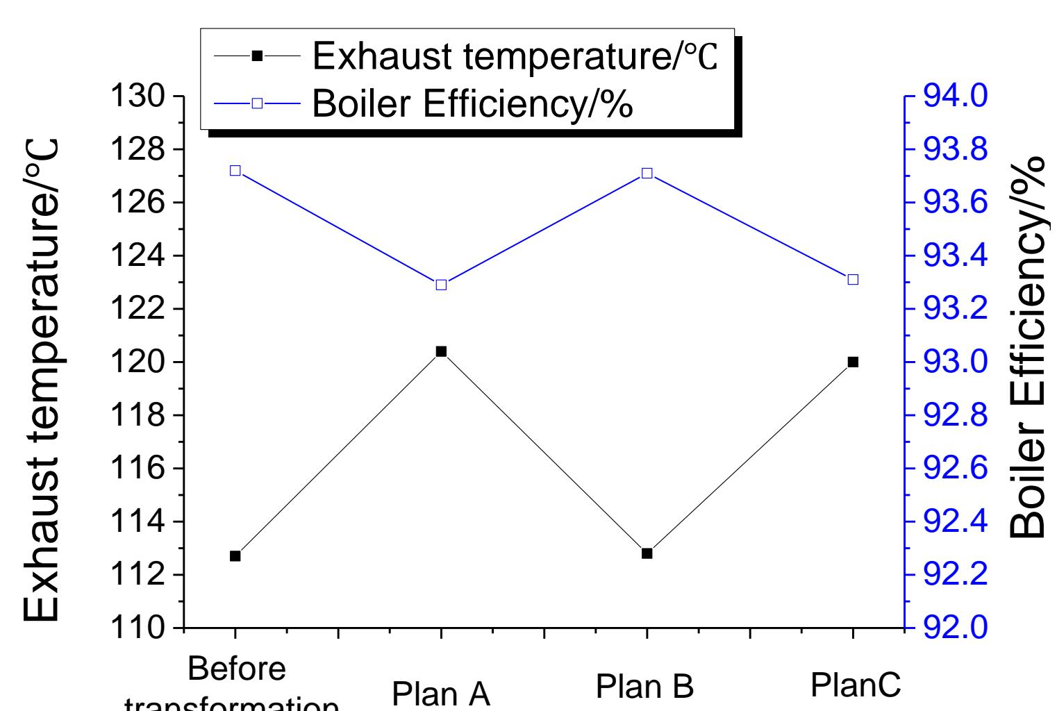
Finally, the program C flue gas bypass modification program is selected for wide-load denitrification modification. After the transformation, under ultra-low load conditions, the inlet flue gas temperature of the SCR can be increased to over 300°C through bypass flue adjustment, and at the same time, the safety and economy of the unit under high load conditions will not be affected.
