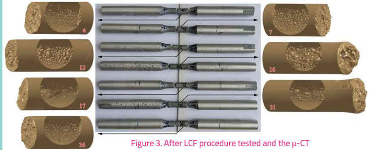
Figure 3. After LCF procedure tested and the \mu -CT scanned specimens.
