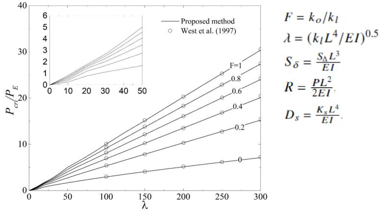
Variation in critical load for a free-free pile. F=0 (triangular linear distribution of  $k_s$  and F=1 (uniform distribution of  $k_s$ )
