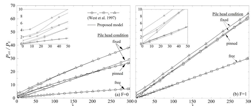
Critical load for a pile in a soil with (a) F=0 and (b) F=1 and various end-boundary conditions. ( $\triangle$ ) fixed; ( $\bigcirc$ ) hinged; and ( $\square$ ) free.
