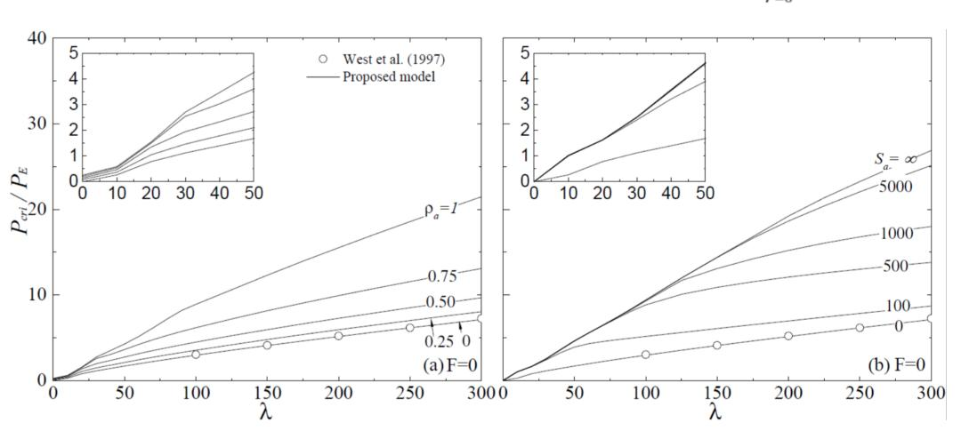
Effects of a (a) rotational and (b) translational restraint at the pile head on the critical load for a pile free at the bottom and embedded in a soil with F=0.
