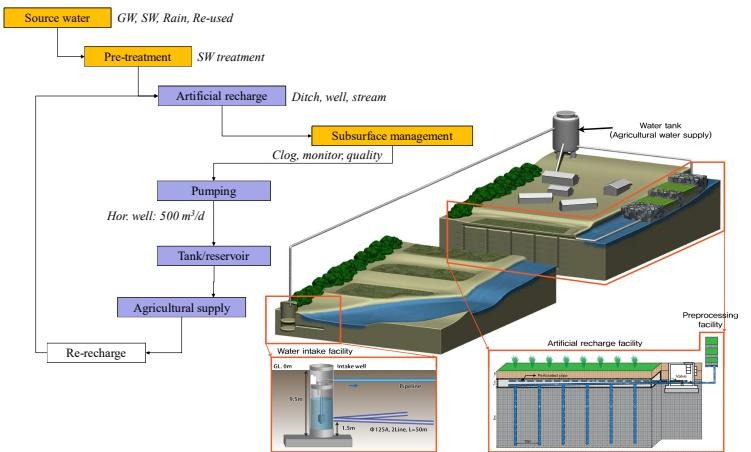
**Artificial recharge facility :** 2 trench lines on the right side of the recharge area (80m), 2 trench lines on the left side of the recharge area (100m)
