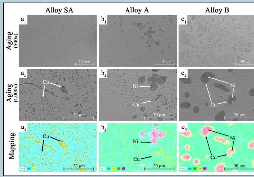
Figure 5. SE microstructure images and mapping of aging alloy. a) Alloy SA shows the segregation of Cu second phase b) Alloy A shows Ni second phase precipitated and cu scattering into the matrix c) Alloy B Ni second phase precipitate and cu phase wrap
