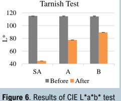
comparison before and after tarnish test of alloy SA, alloy A, and alloy B
