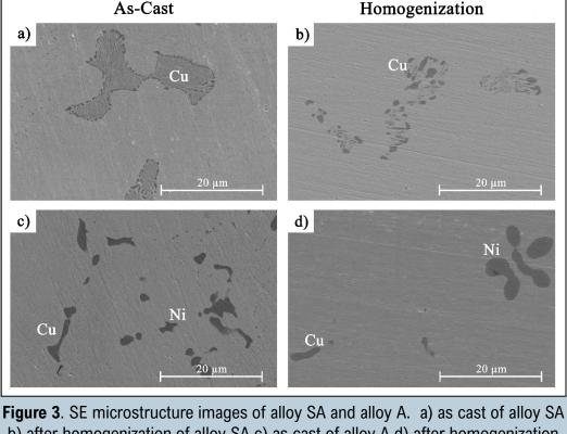
b) after homogenization of alloy SA c) as cast of alloy A d) after homogenization of alloy A
