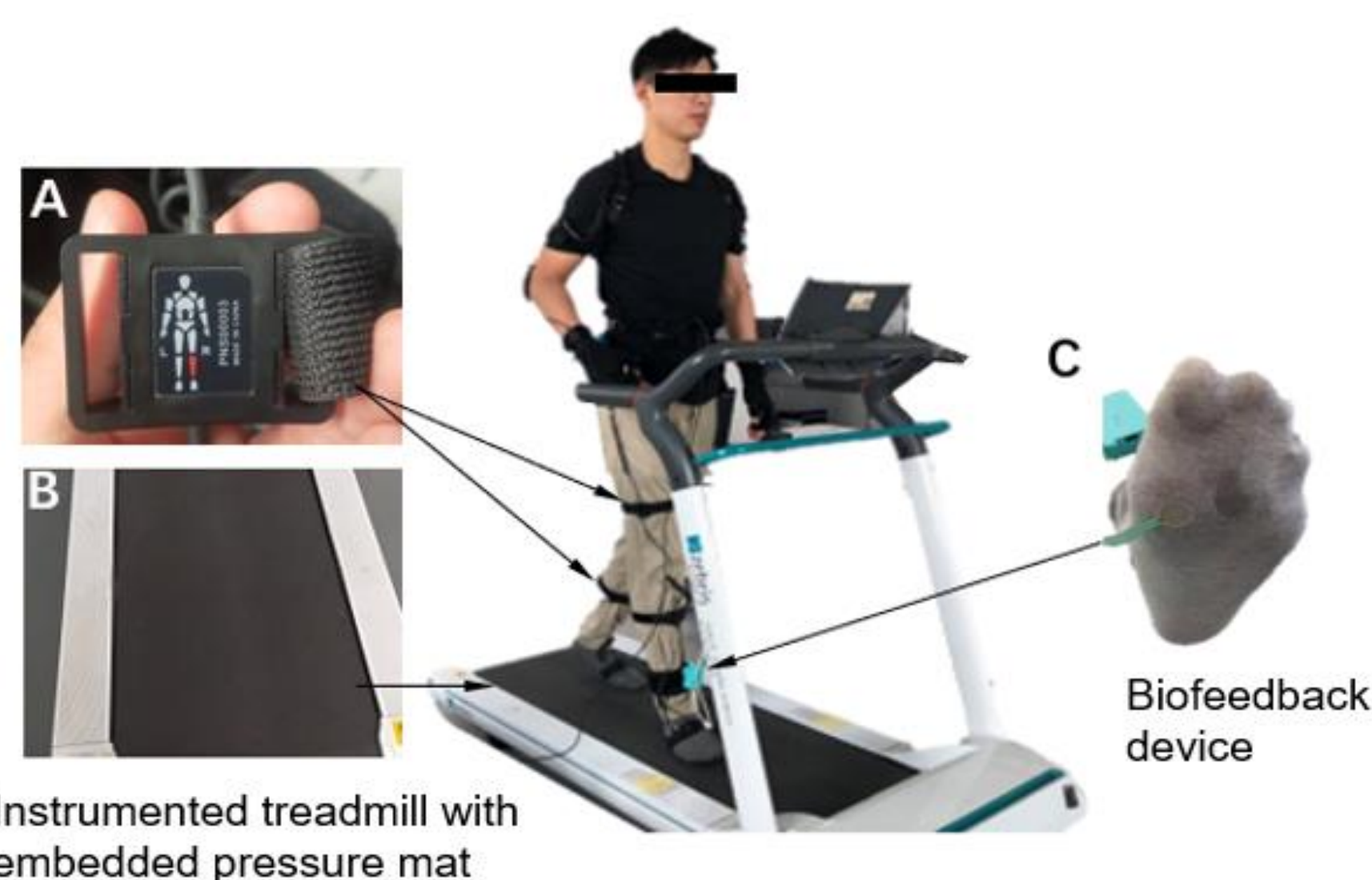
Figure 1. Experiment setting for simultaneous acquisition of lower extremity joint kinematics and dynamic plantar pressure distribution during biofeedback-assisted gait training
