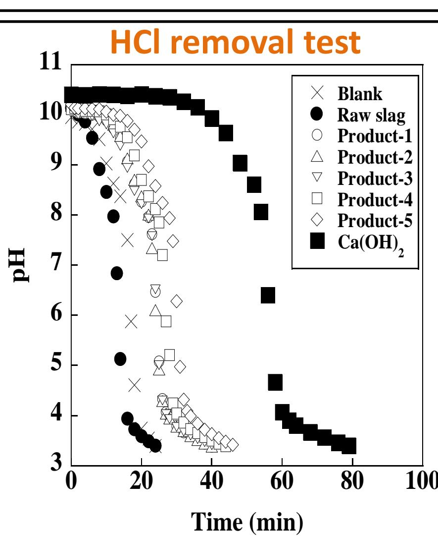
Fig. pH of the solution with dissolving HCl gas after passing through raw slag,  $Ca(OH)_2$  and the product.
